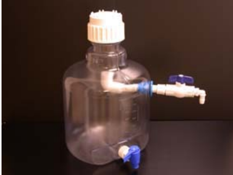
Figure 3. Paramecia collector. The paramecia collect at the top of the carboy and are then removed by the pipe fittings near the top. The collector is made from a carboy with a spigot at the bottom and a modified suction drain (see figure 4). A four gallon carboy is recommended for larger facilities, while a 2 gallon carboy will work well for those needing only small amounts of paramecia.
