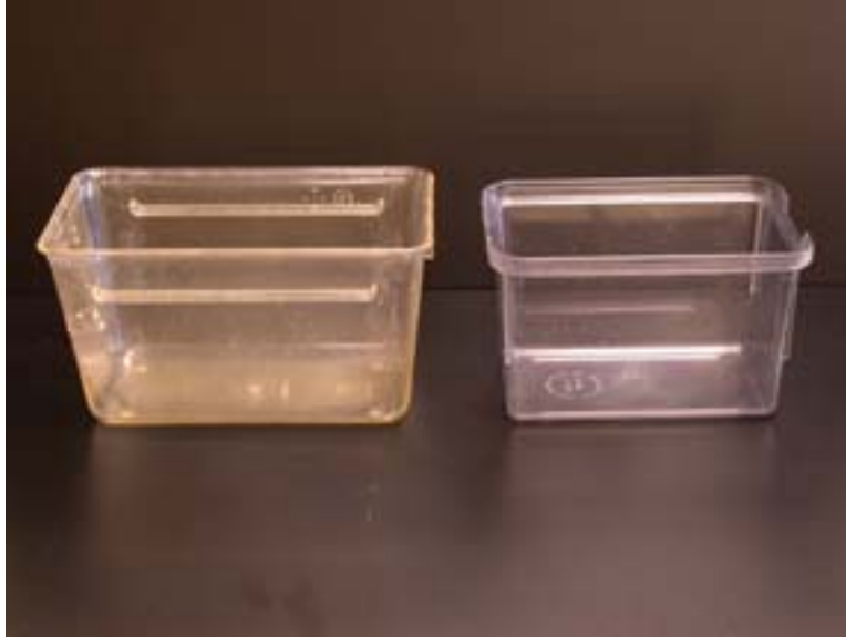
Figure 1. Examples of sub-culture containers ranging in size from 500 to 2000ml. The container on the left is a polycarbonate Nalgene animal cage (24x14x13cm). It has a volume of approximately 2 liters. The container on the right is a Thoran crossing cage and holds approximately 1 liter.
