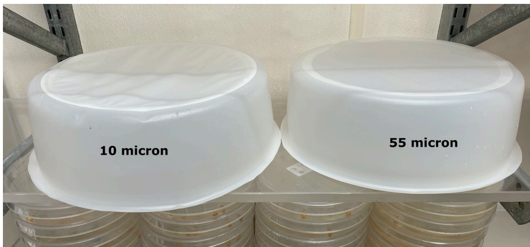
Figure 2. Mesh sieves used in the cleaning and concentrating of paramecia. A 10 \mu\text{m} and 55 \mu\text{m} EZ-Strainer can be obtained from various on-line vendors. To speed the sieving process, a large sieve diameter is recommended. See vendor information below or contact, zirc@zebrafish.org for questions.
