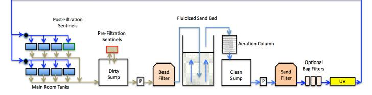
Water source is reverse osmosis treated municipal water with added salt and aragonite. 10-12% water exchanged per day.
