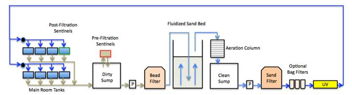
Water source is reverse osmosis treated municipal water with added salt and aragonite. 10-12% water exchanged per day.
