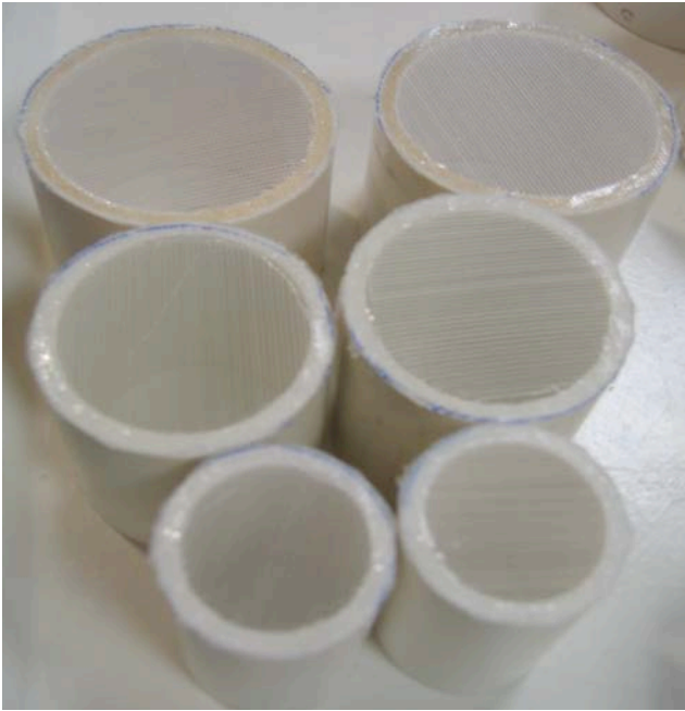
Fig 1. Mesh baskets. Made by using hot glue to adhere nylon mesh (~500 microns) to the bottom of PVC pipe. Various sizes can be made to hold larger amounts of eggs.
