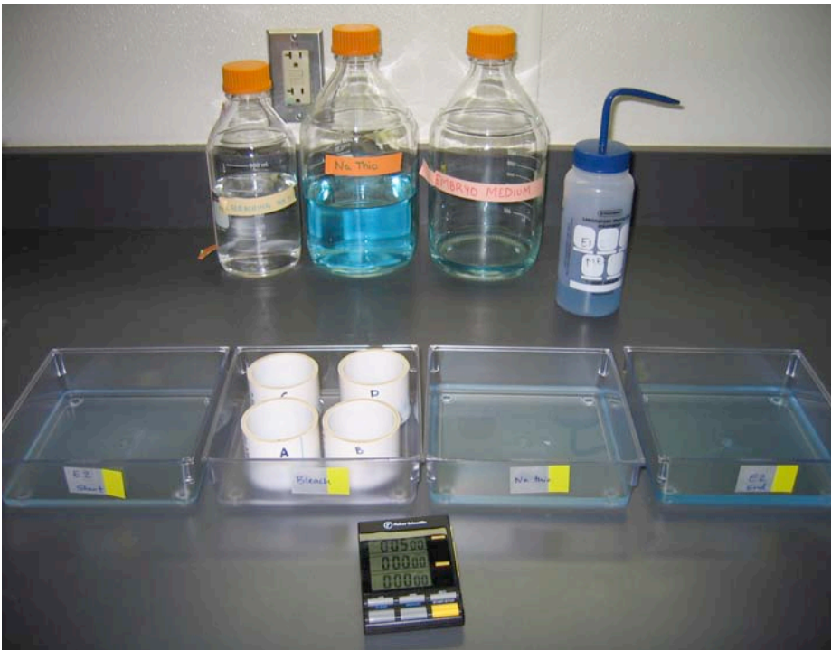
Fig 2. Egg bleaching station. 4 containers are set up for bleach, sodium thiousulfate-pronase, and rinse solutions. Pre-made large volume solutions are shown in the background.
