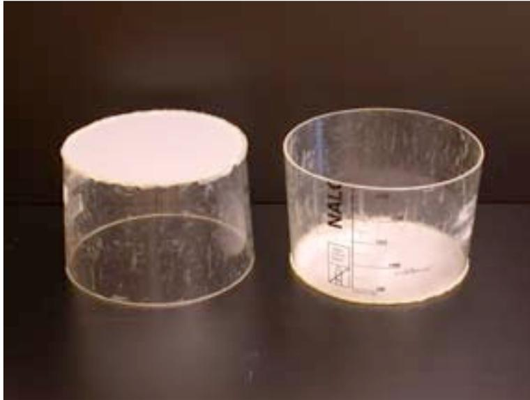
**Figure 2.** Strainers used in the cleaning and concentrating of paramecia. The strainers are hand made by taking a large plastic beaker and cutting it into cylinders. Polyester filter or bolting cloth is then fixed to one side using hot glue. 10  $\mu\text{m}$  and 105  $\mu\text{m}$  mesh sizes.
